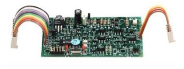
System Sensor Protocol Loop Driver Card for Morley ZX range of Analogue Addressable Fire Alarm Panels. One loop card needs to be ordered per loop.
