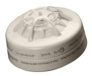
The Orbis IS Heat Detector monitors temperature by using a single thermistor network which provides a voltage output proportional to the external air temperature. The Orbis IS range incorporates seven heat detector classes to suit a wide range of operating conditions.
