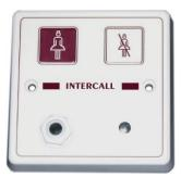
A call point is needed for every individual call location on the system. Every L622 unit features five levels of call, multi-colour reassurance LED alerts and a 'call follower' sounder. The jack socket accepts inputs from a wide range of triggering devices such as pear leads, pressure mats and portable radio triggers. A magnetic reset option is also available (order code L622M) which only allows the reset function to be activated by the use of a magnetic key.
