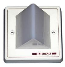
These are normally positioned above doors in a corridor to indicate the status of the call point(s) within each room. The L746 can also be used to monitor several call points for end of corridor indication, or as a 'follow me' light. Each unit is fitted with twin ultra-bright LEDs which mimic the reassurance indicator on the call points. Also available with an integral sounder alarm (L746S).
