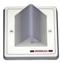
These are normally positioned above doors in a corridor to indicate the status of the call point(s) within each room. The L746s can also be used to monitor several call points for end of corridor indication, or as a 'follow me' light. Each unit is fitted with twin ultra-bright LEDs which mimic the reassurance indicator on the call points. The sounder mimics the LCD display sounding patterns.
