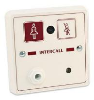
Specifically developed for bathrooms, toilets and other areas where the intercom facility is not require. The L722 is a Non-Audio call Poin, which incorporates 3 levels of call, Standard, Assistance and Emergency. The unit also features an infra red receiver and reassurance LED.
