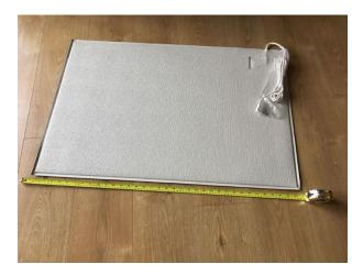
The large anti-bacterial pressure mat is placed on the floor and simply connects to your nursecall system activating a standard call when a resident steps on it. The unit comes with a 2.5 metre lead and plugs onto the call unit jack socket. The mat measures approx. 610 x 910 mm. A smaller standard version is available.
