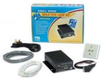
Hearing loop systems allow hearing impaired people to hear more clearly. Most hearing aids have a 'T' or 'MT' switch which allows them to pick up the electromagnetic field generated by a hearing loop system. The hearing aid converts this signal into a sound suited to its user's specific hearing requirements.
