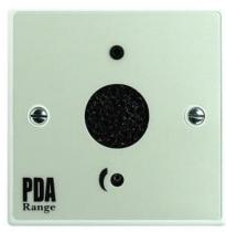
The Outreach Plate audio input extension system comprises a range of wall, ceiling and desk mountable plates specifically designed to increase the audio input capability of any audio system. Covering the most common variants of audio connectors, they work by mixing the signals from various audio input sources into a single balanced line level input on a compatible amplifier. Each input plate features a built-in mixer, preamp, input level control and balanced output.
